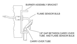
FIGURE 21 - PROPER FLAME ADJUSTMENT
