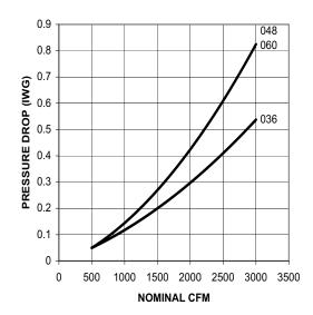
FIGURE 17 - PRESSURE DROP ACROSS COIL
