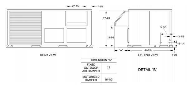
FIGURE 13 - UNIT WITH FIXED OUTDOOR AIR/MOTORIZED DAMPER RAINHOOD
