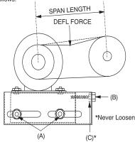
Tension new belts at the max. deflection force recommended for the belt section. Check the belt tension at least two times during the first 24 hours of operation. Any re-tensioning should fall between the min. and max. deflection force values.
