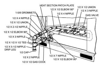
FIGURE 5 - BOTTOM SUPPLY CONNECTION EXTERNAL SHUT-OFF
