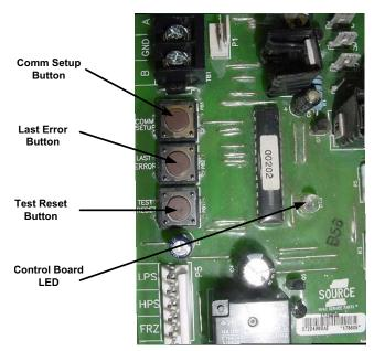
FIGURE 26 - UNIT CONTROL BOARD
