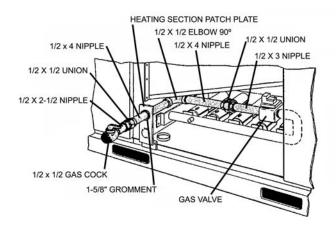
FIGURE 4 - EXTERNAL SUPPLY CONNECTION EXTERNAL SHUT-OFF
