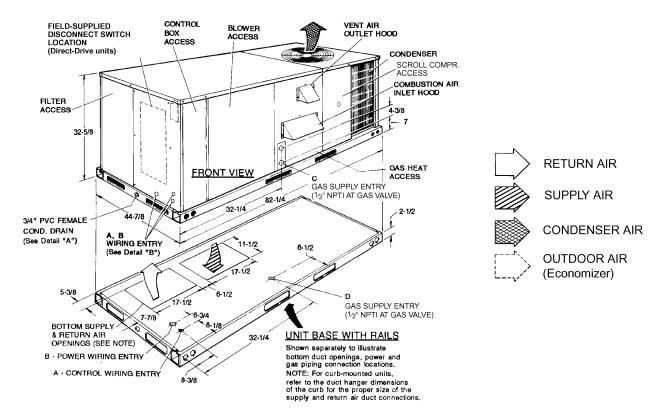
FIGURE 11 - UNIT DIMENSIONS (3 - 5 TON COOLING/GAS HEAT) FRONT VIEW
