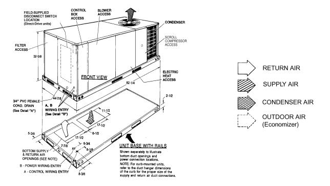
FIGURE 10 - UNIT DIMENSIONS (3 - 5 TON COOLING ONLY/ELECTRIC HEAT) FRONT VIEW
