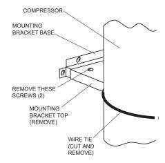
FIGURE 2 - COMPRESSOR RESTRAINING BRACKET
