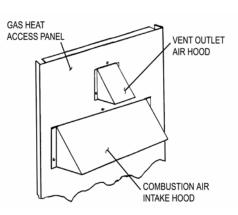
FIGURE 6 - VENT AND COMBUSTION AIR HOOD
